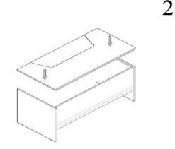
Top tray is placed on the stand and the cover and the minifixes are tightened by the help of a screwdriver.
