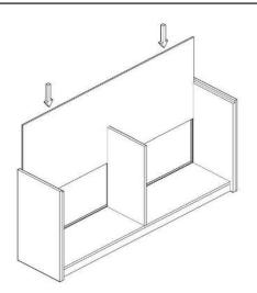
The backboard is inserted into side trays and backboard channels opened on the bottom tray.
