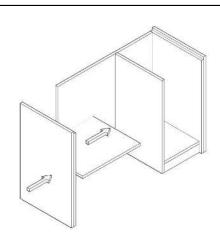
The stable baffle is placed on the spaces in left side respectively and their minifixes are tightened with the help of a screwdriver.
