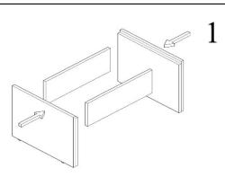
Minifix shafts located on the stands precisely placed on the minifix heads located on the bases and tightened with the help of a screwdriver.
