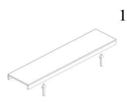
Base parts are placed on the lower part of bottom tray. Minifixes are tightened with the help of a screwdriver.
