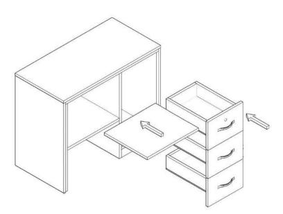
1 piece of rail is included in the keyboard package. There are sign holes on the left side tray and on the left side of mid-tray for connecting the rail. The rails are connected by using a 3.5 \* 18 screw. The other parts of the rails are connected to the keyboard tray. The keyboard and drawers are put in their places. The handles are fixed to the drawer tabs by using 22mm button-head handle screws.
