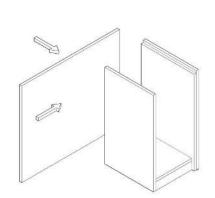
The 18mm back tray is fixed to the side trays and to the bottom and top part with minifixes.
