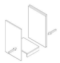
The right-side tray and mid-tray are placed on the spaces located in the bottom tray and the minifixes are tightened with the help of a screwdriver.
