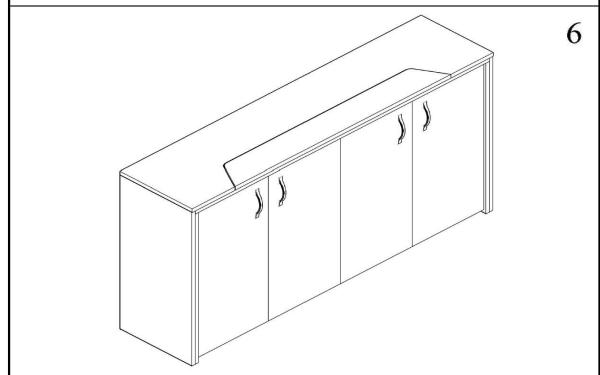
The doors are connected to the side trays and the pillar with 3.5 \* 18 screws. Super camel hinge is used for outer doors and half camel hinge is used for inner doors. The handles are fixed to the lids by using 22mm button-head handle screws.
