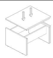
The top tray is placed on the stands and the minifixes are tightened with the help of a screwdriver.
