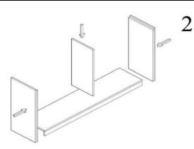
The side trays are placed on the spaces located in the bottom tray and the minifixes are tightened with the help of a screwdriver.
