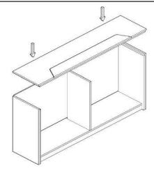
Top tray is placed and the minifixes are tightened with the help of a screwdriver.
