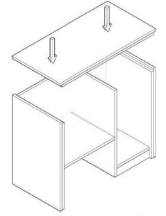
Top tray is placed and the minifixes are tightened with the help of a screwdriver.
